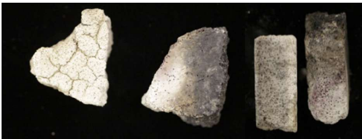
Figure 15.3.1: Example of burned sheetrock. Burned sheetrock used as building material appears similar to human bone but can be differentiated by the fact that it is the same density throughout.
