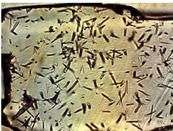
Figure 7.5.6: Thin section showing damage tracks from fission.
